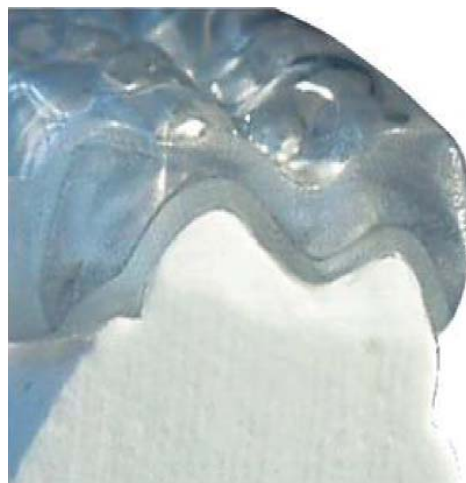
Figure 1. Cross section of formed PETG/PU material - note proportions of soft layer (facing the fitting surface) and the hard layer (facing the opposing dentition).
